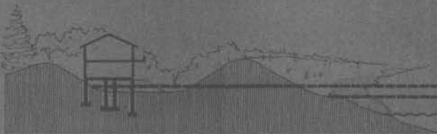
The addition of fill material can impede the flow of flood water and may increase flooding levels, thus causing damage to buildings previously above the BFE.
