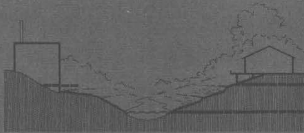
Buildings in a riverine setting should be located above the Base Flood Elevation (BFE).
