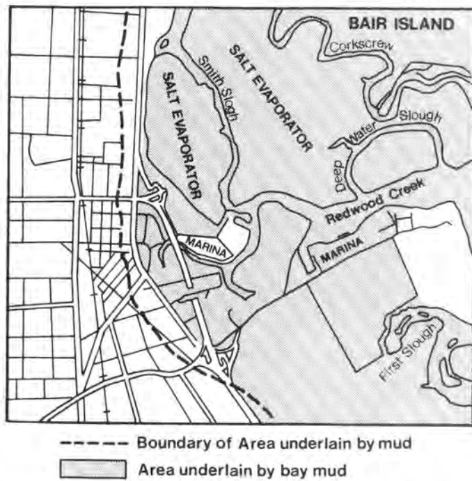
Figure 9-4. Part of a map showing the area of Redwood City, CA underlain by bay mud. The map is attached to the building code which requires supplemental structural design and construction standards for all new development. Source: U.S.G.S.
