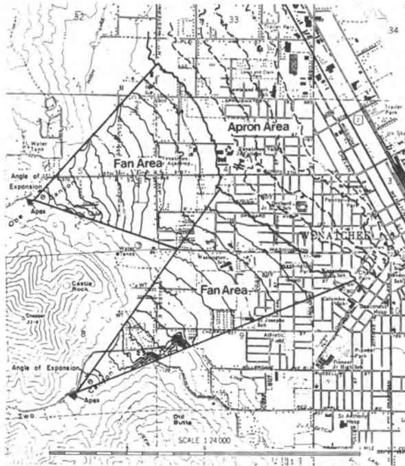
Figure 3-3. Topographic characteristics of typical alluvial fans and alluvial aprons (Wenatchee, Washington). Source: FEMA.
